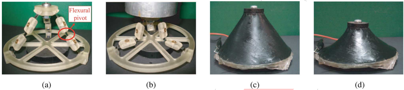
Fig. 2. Actuator prototype. Frame prototype in (a) undeflected condition and (b) under constant external load application, actuator in (c) deactivated and (d) activated states.
