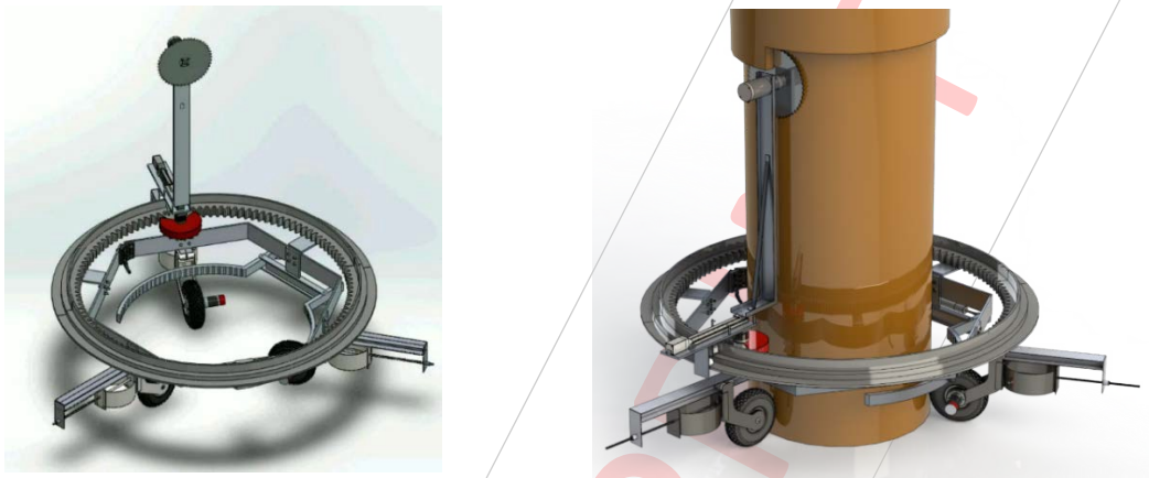
Figure 3. Overall 3D view of ACROBAT: resting position (left) and performing a pruning operation on a palm trunk (right).
