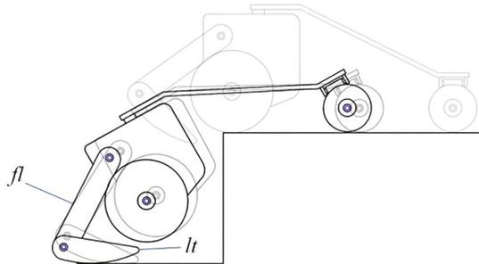
**Fig. 3.** During the step descent the rotating leg tips realize shock absorption.
