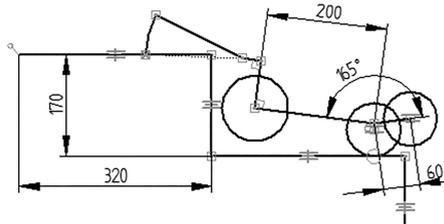
Fig. 4. Main geometrical parameters of the six-wheeled rear carriage.
