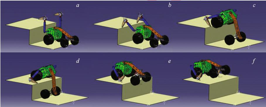
**Fig. 2.** Maximum pitch angle with 4-wheeled rear carriage.
