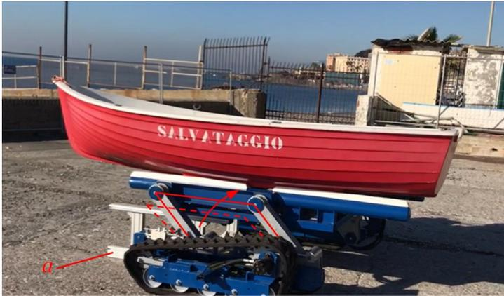
**Fig. 2.** Elloboat relieving a boat from a fixed support (a) by lifting the saddle.
