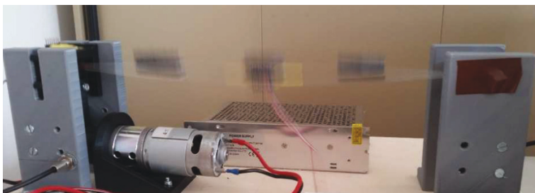
Fig. 5. Forced vibration of flexible beam - input frequency close to resonance frequency.
